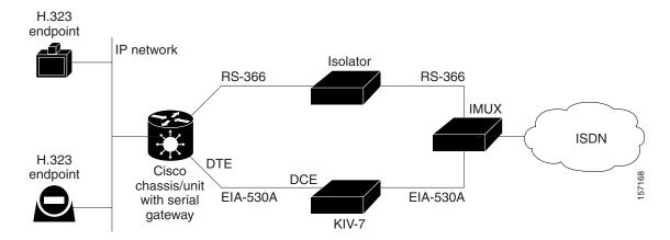
Figure 1-7 Encrypted Videoconferencing via Satellite
